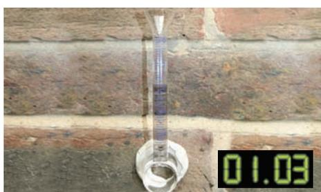
Continue to monitor the water level at regular intervals - preferably for at least one hour. The results can be plotted on a graph using the template overleaf.
