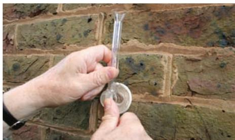
Press the Stormdry Gauge firmly onto the masonry to be tested. Ensure the Gauge is upright, and a good seal has been made with the masonry. It can be affixed to brick, over a mortar line, or to stonework.
