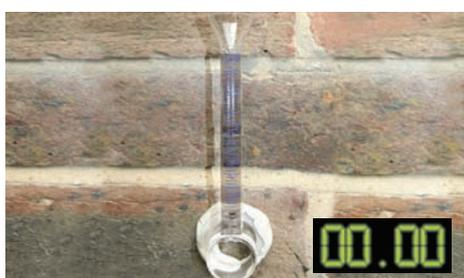
Start timing as soon as the gauge is filled. Keep a check on the water level to see if it drops. For highly absorbent surfaces this will be easily apparent within a few minutes.
