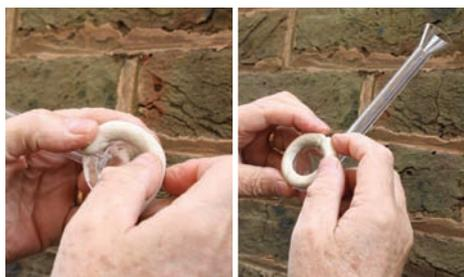
Ensure the flange of the Stormdry Gauge is clean and dry, and then apply mastic adhesive. Complete an "O" ring of adhesive, ensuring there are no air gaps.
